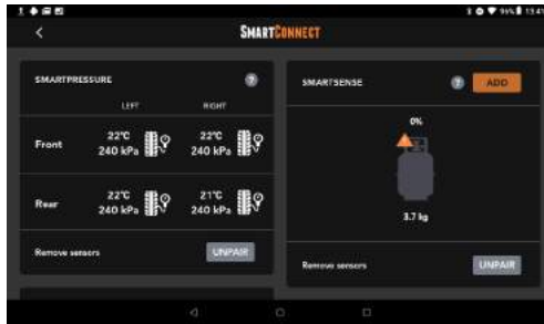
Figure 17: SmartPressure sensors icons after successful pairing
