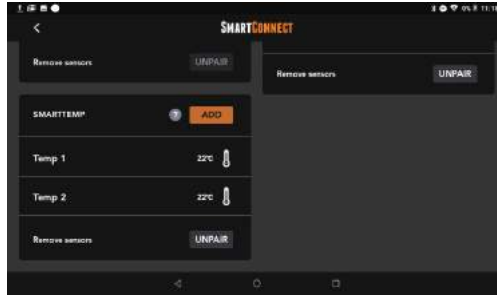
Figure 20: Adding a SmartTemp Temperature Sensor
